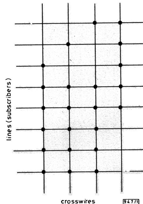
Fig. 1 An R2BSN(4) with minimal switches
